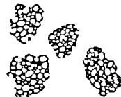
c) AGGLOMERATES ARE FORMED BY BINDING FINES TOGETHER AFTER MODIFYING CLAY PROPERTIES, LIME AND PORTLAND CEMENT CAN BE USED.
