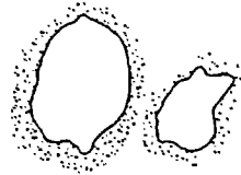
a) FINES ARE AGGLOMERATED ONTO COARSE PARTICLES, BINDER SUCH AS PORTLAND CEMENT IS USED.
