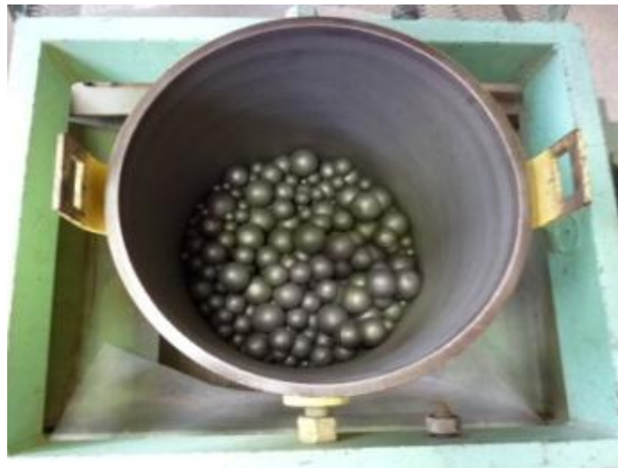
Figure 10 –balls distribution and jar used for Bond Work Index assessment tests
