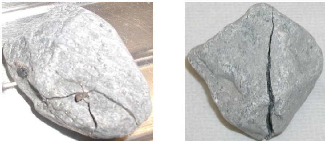
Figure 13 – Pebbles fragmentation linked with fast temperature rise during microwaves treatment
