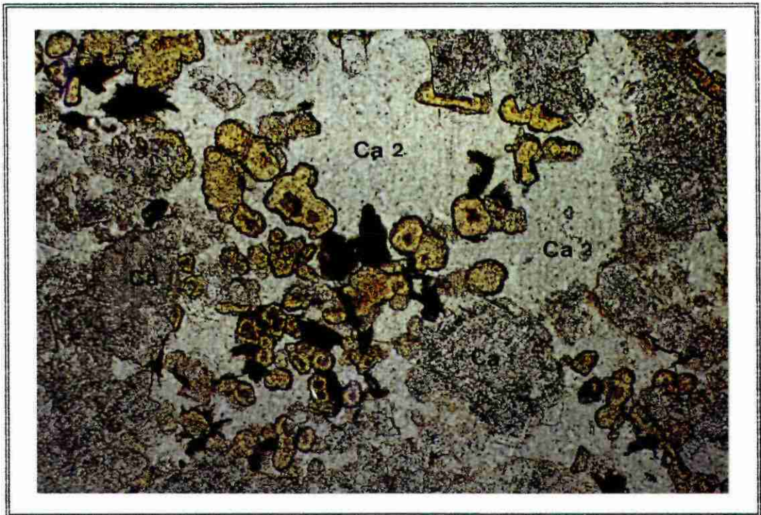
Fig. 13: Zoned REE-minerals (yellowish), with dark cores which are very rich in Ce (possibly Ce-bastnaesite, fluocerite or cerium oxide) and paler P-Sr-rich margins (possibly belovite, see chap. 3.4.2).
