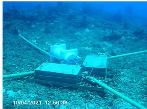
Figure 1: STATEM magnetotelluric instrument
