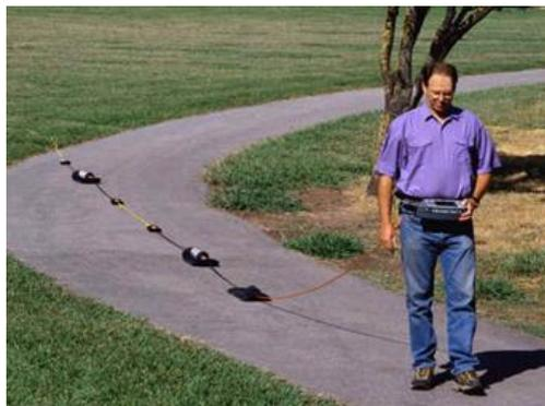
Figure 10 - OhmMapper (source Géometrics).
