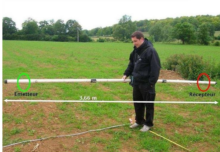
Figure 9 - Géonics EM31 (source Polytech'Paris-UPMC).
