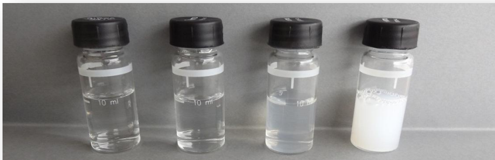
FIGURE 9 : ETALONS DU TURBIDIMETRE HI 98712 (0/15/100/750 NFU)
