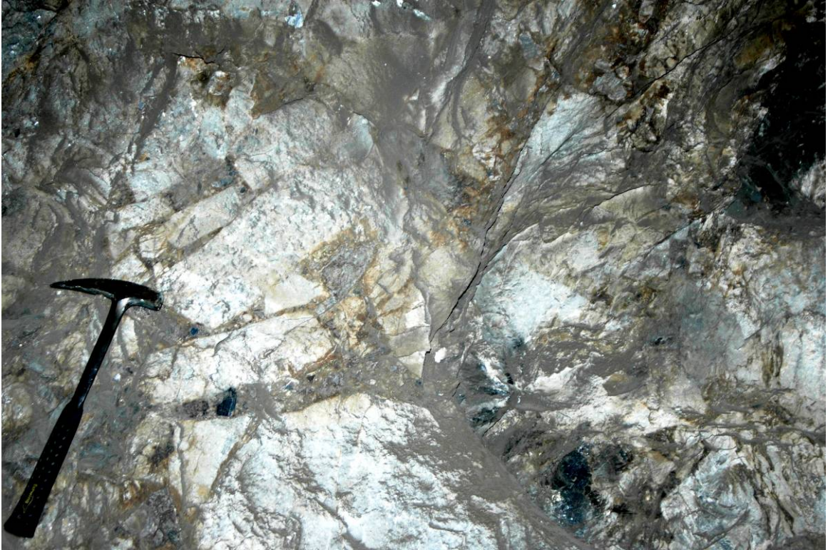
Photo 5 - Hydraulic breccia in marmorised limestones hosting the mineralisation, close to the volcanic breccia. To the right of the handle of the hammer, smashed schists fragments (in black), clay, phyllites and minute fragments of dacite constitute the matrix
