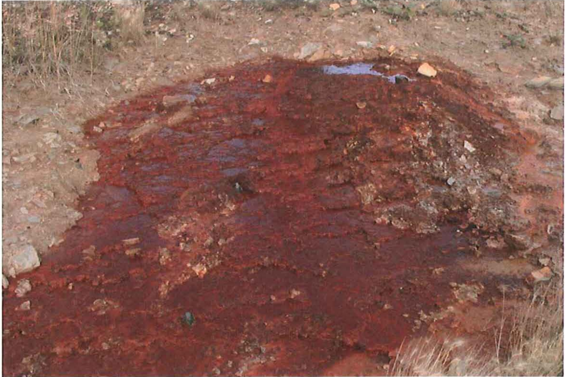
Illustration 13: "acid spring" flowing out the dumped Cypris material (observation point SO 6)
