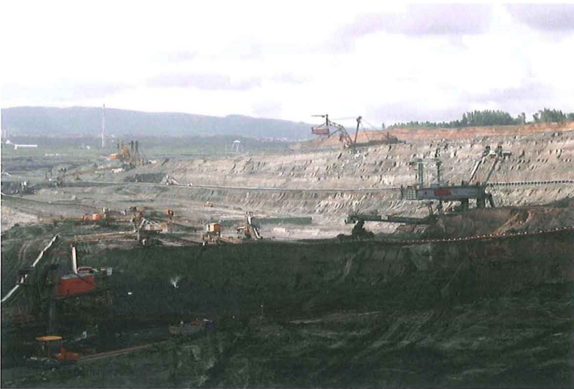
Illustration 6: bench-type exploitation of the lignite at the Jiří mine
