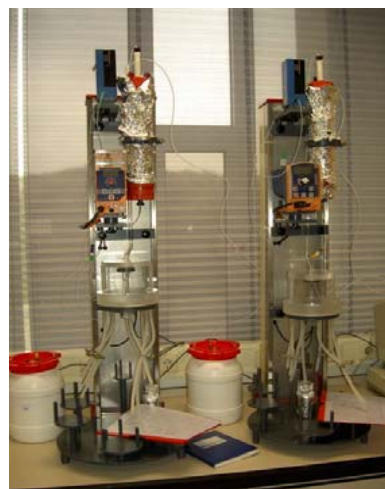
Automated pH-static (TS14997) and percolation (TS 14405) test
