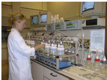
Automated pH-static (TS14997) and percolation (TS 14405) test
