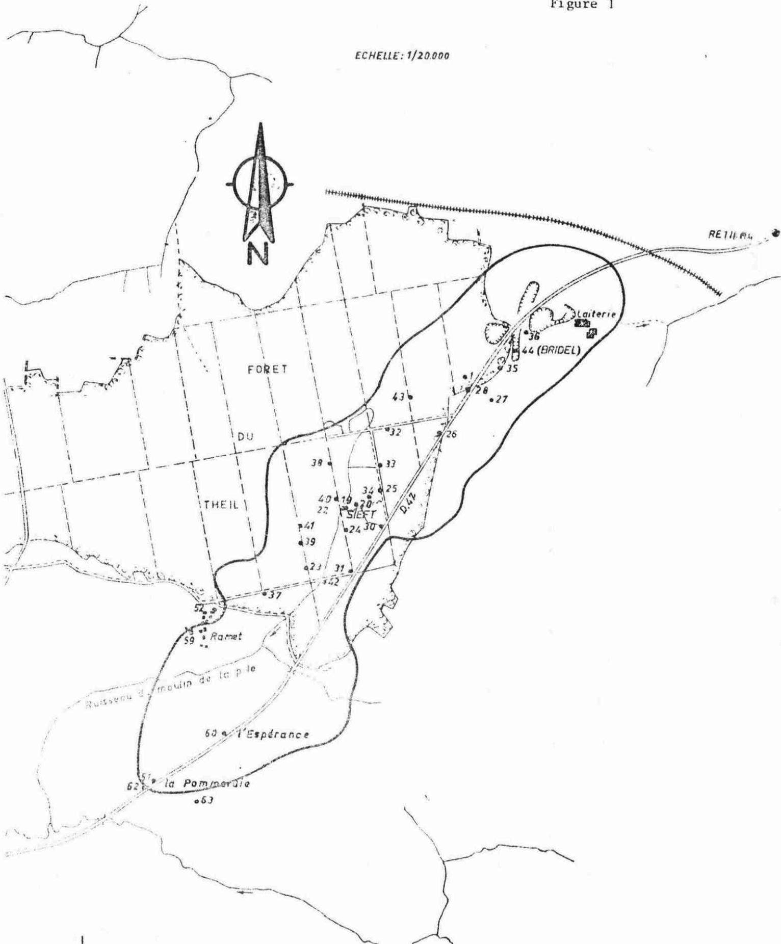
1 - MESURES PIEZOMETRIQUES - FLUCTUATIONS DE LA NAPPE
