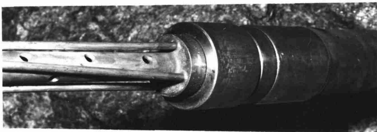
b) Introduction of the piezopermeameter into a borehole
