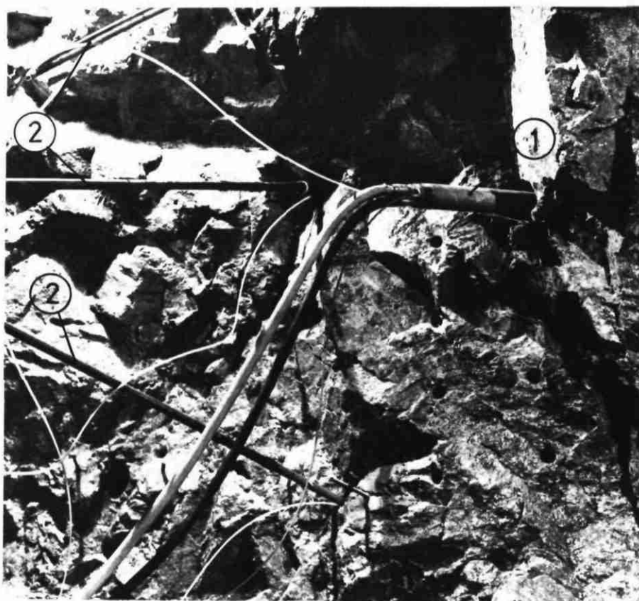
Fig. 10 - Examples of testing with the triple hydraulic probe (1) Triple hydraulic probe (2) Lateral piezometers (3) System to move the probe.
