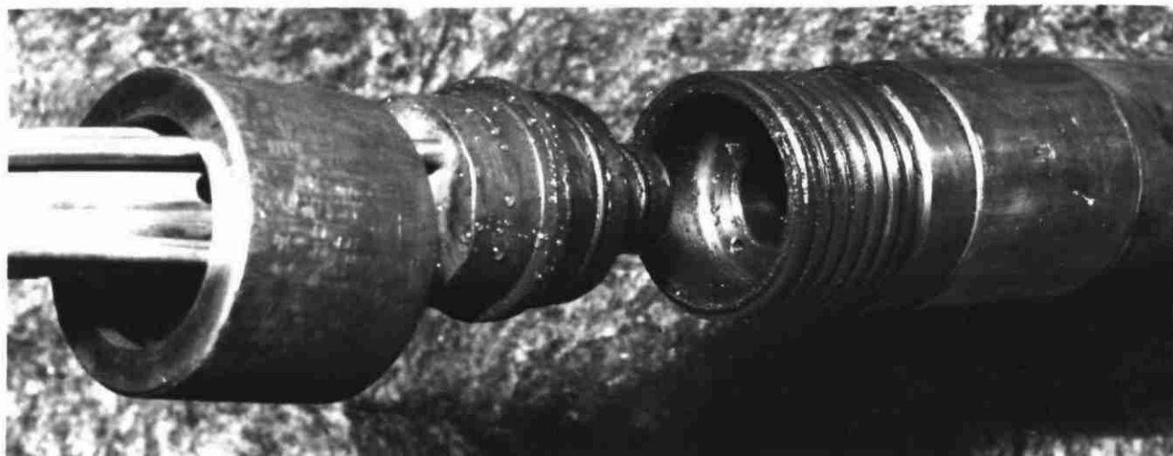
a) Coupling the screen with the generalised pneumatic packer
