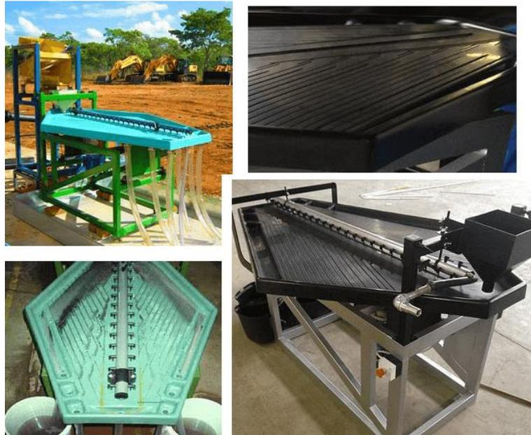
Figure 39 : photographie d'une table à secousses Géméni ([https://www.911metallurgist.com/blog/gemini-gold-shaking-table#lightbox\[postimages\]/0](https://www.911metallurgist.com/blog/gemini-gold-shaking-table#lightbox[postimages]/0))
